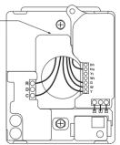
Some installations have limited wires between the thermostat and the HVAC equipment. The included Wiring Module can be used to control the HVAC equipment without having to run new or additional wires to the thermostat.
