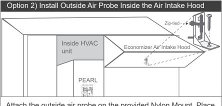
Attach the outside air probe on the provided Nylon Mount. Place mount inside the air intake hood where sun and water will not affect temperature readings.
