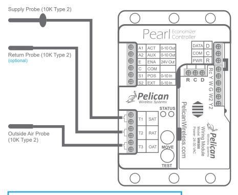
CAUTION: The Outside Air Temperature Probe must be mounted outside in a weather resistant, sunsheilded enclosure or inside the air intake hood mounted on the provided nylon mounting stand.
