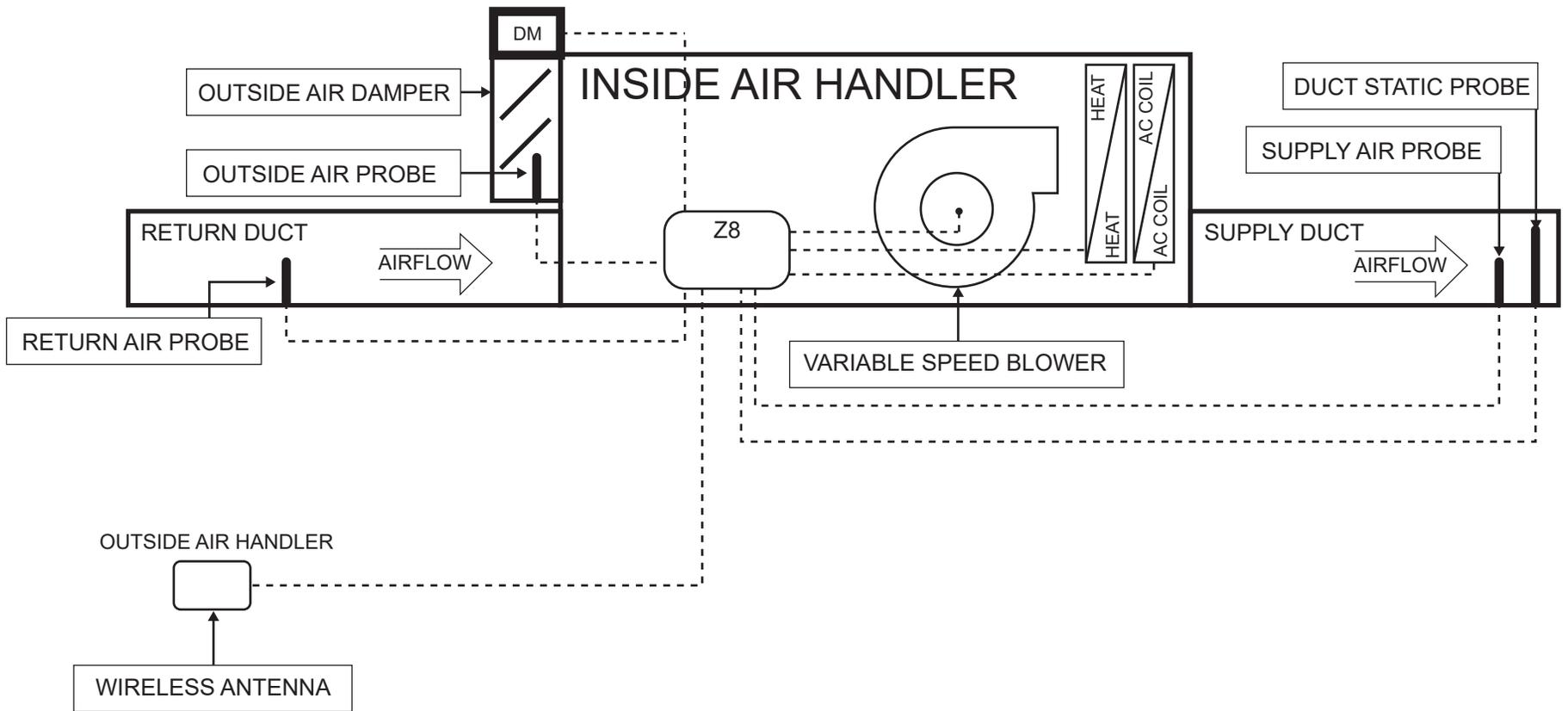
REFER TO PELICAN Z8 INSTALLATION GUIDES FOR CONTROL TERMINAL WIRING AND SEQUENCE GUIDE
