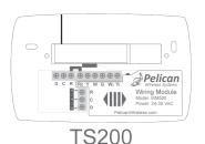
**Step 2:** Loosen R and Rc terminals and remove jumper. Loosen R, C, D terminals on Wiring Module. Slide Wiring Module to the right to remove.
