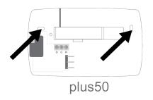
**Step 5**: Install Wiring Module into plus50 sub-base. Install jumper between R and Rc. Tighten R and Rc terminals. Tighten R, D, C terminals on Wiring Module.
