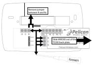
**Step 3:** Remove existing TS200 or TS200H sub-base from wall.
